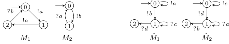
Fig. 2. Examples of AD (left) and non-AD (right) systems.
